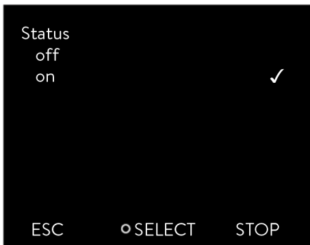
Fig. 12: Flow controller off/on
