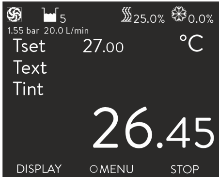
Fig. 9: Basic window of Integral XT and Integral P with flow controller
